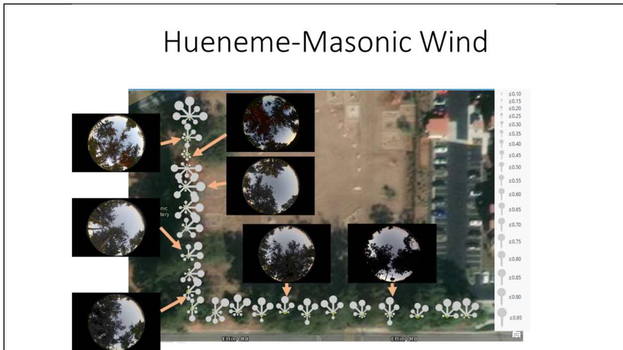
Figure 4c. Wind “Roses”. A wind rose is a circular display of how wind speed and direction are distributed at a given location for a certain time period. The size of the “petal” equates to the speed of wind from that direction. The larger the “petal” means there is more wind coming from that direction. Smaller “petals” mean there is more wind protection in that direction.
